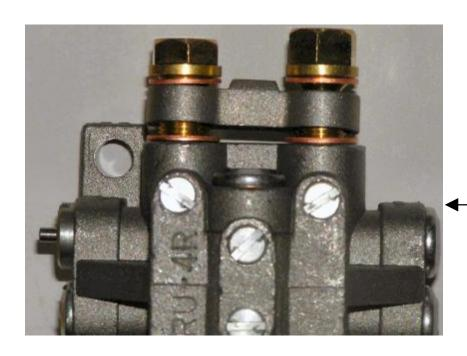
The connector installed (loosely) on the block.
