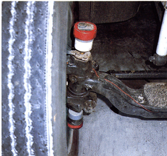
SEMI-TRAILER FRONT END KINGPINS
